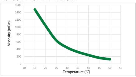
Test specimens were neat epoxy (without fibre reinforcement). Typical values not to be construed as specification.
